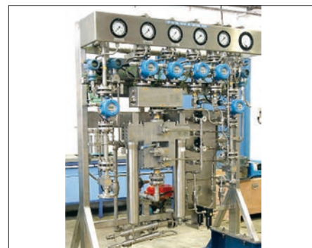
Filter station for the filtration of gases with STAUFF-3-way-selector ball valves for 250 bar / 3600 PSI and +200°C / +392 °F.
