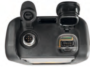
PPC-04-plus-CAN with CAN interface for max. 3 sensors (max. 50 m / 164 ft cable length)
